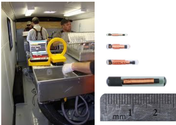
Figure 3- Left- An example of a pit tag reader (yellow circle). Left- Examples of the different sizes of pit tags used for various fish species.
